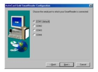
Usually, you connect the Smart Reader on COM1 and the Keyboard connector.
