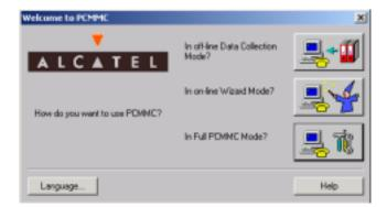
Click on Full PCMMC Mode and start with local Online Connection Mode. You have to have the console cable connected to "system" DB9 connector. The switch close by needs to be set to local. The cable type is 1:1
