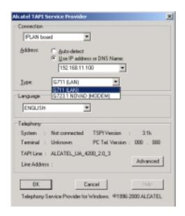
You also could use this application with use of a modem attached to your PC, but this is not the purpose of this setup. Don't change any settings on Advanced Button, as the default setting are mostly OK. The set to do is click on OK in the window above and a new window comes up with Setup Complete. Click on Finish and you are set.
