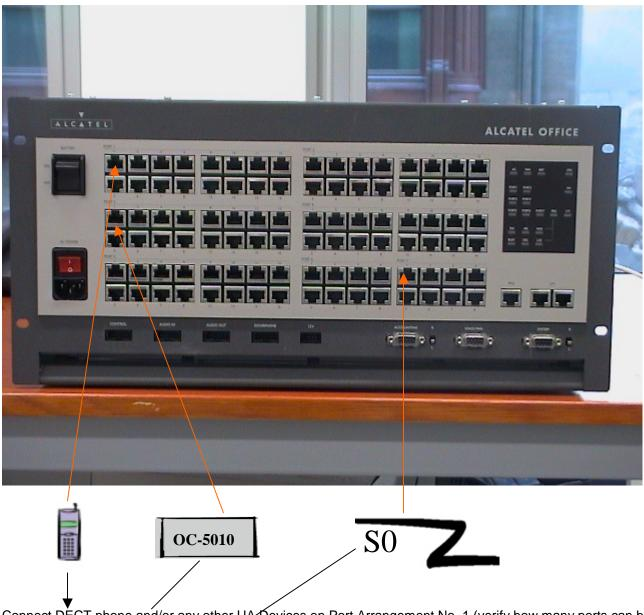
Connect DECT phone and/or any other UA Devices on Port Arrangement No. 1 (verify how many ports can be use, for example DLC8 can only provide outlets (RJ-45) one to eight
