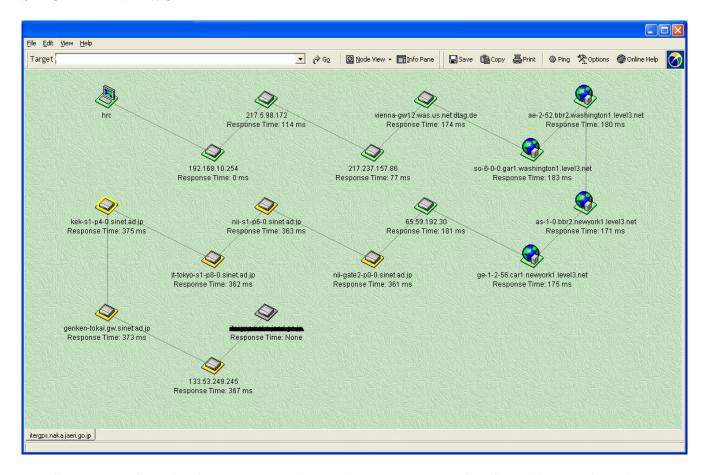
My client "HRC" did a visual trace to a host, located in Japan. Because of the long delay, the throughput on FTP is far away from the allocated bandwidth. To setup a test environment, I've used "Dummynet" to add similar latency into my test lab.
